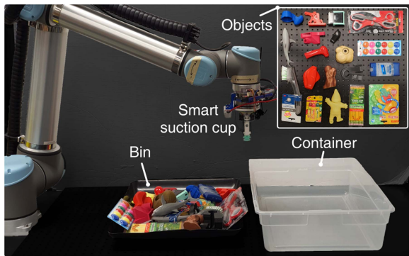
Fig. 8. Tabletop setup for bin-picking experiments. Inset: a dataset of 19 adversarial objects, showing eight 3-D printed objects, six real objects with packaging, and five real objects without a package.
